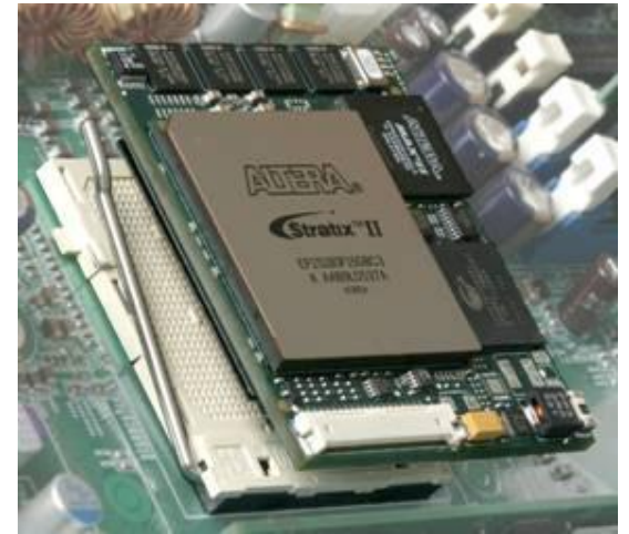
XD1000 FPGA co-processor module for socket 940
