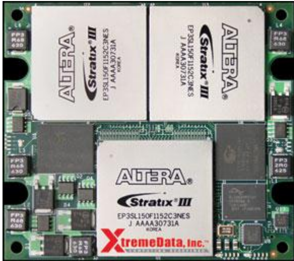
XD2000i FPGA in-socket accelerator for Intel FSB
